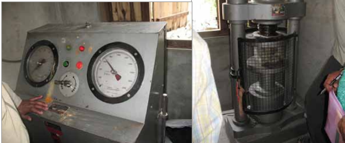
Figure 6: Compressive Strength test of concrete cubes in a local laboratory in Dhangadhi
