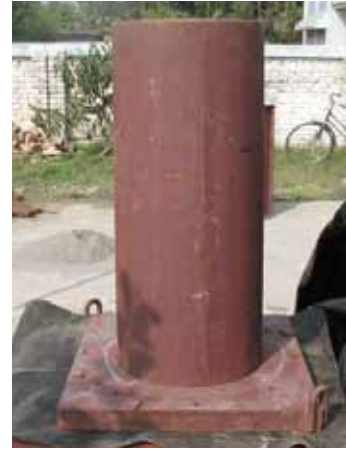
Figure 7: Inner Mould attached with base mould
