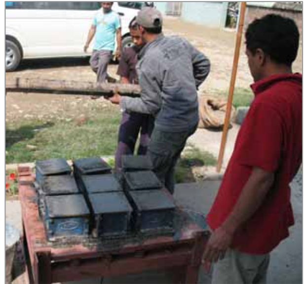
Figure 5: Production of concrete cube in PSU/RVWRMP laboratory, Dhangadhi
