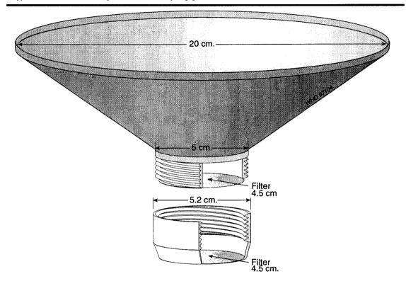
A type of funnel filter widely used for interrupting guinea-worm transmission
