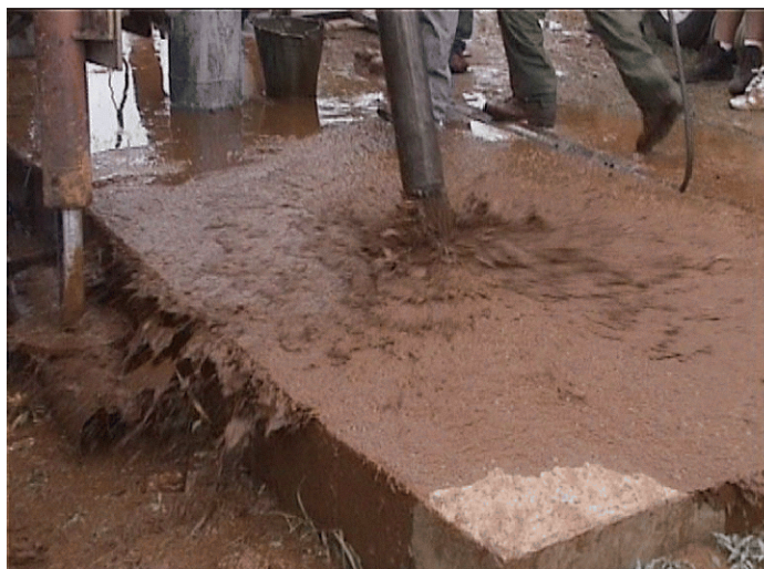
Photo 0: Thick red slime after treatment is a good indicator for heavy iron bacteria attack
