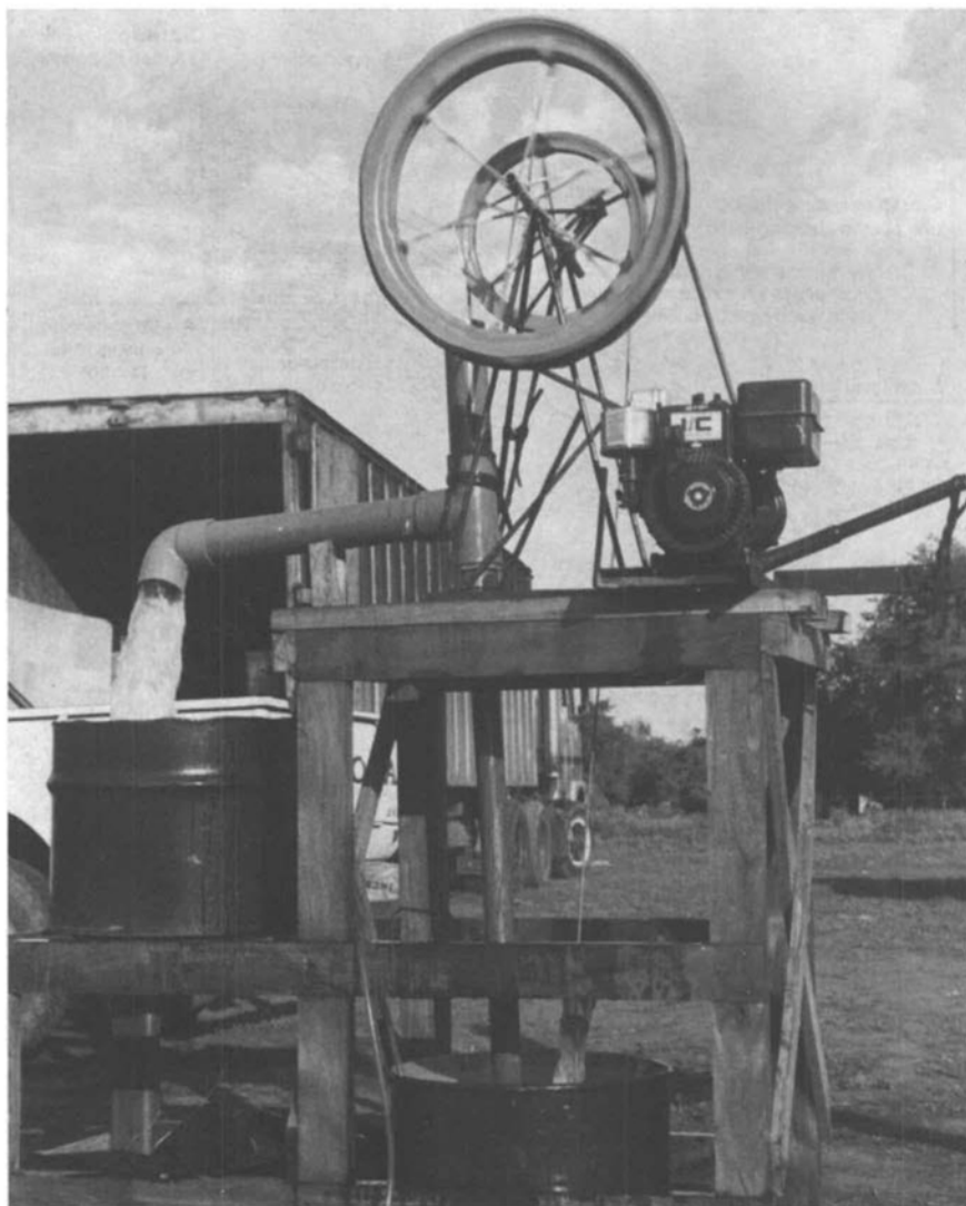
The rope pump can even be attached to a small engine if large quantities of water are needed.
