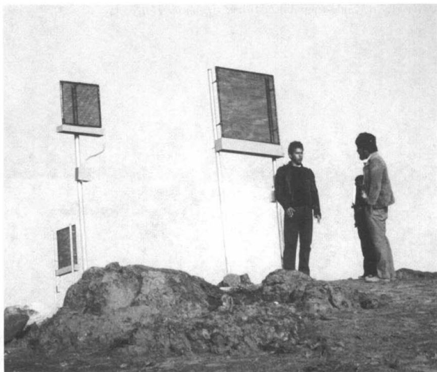
Small fog collectors built to a standard size measuring the fog collection rates at the site in Cerra Orara, Peru.
