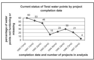
committees, a central maintenance fund and regular fund collection is neither appropriate nor sustainable in the Terai environment. The supply chain for pump spare parts is inadequate and a number of technical issues regarding filters, GI pipes, water quality and platforms have been highlighted. These findings are leading NEWAH to experiment with new innovative approaches.
