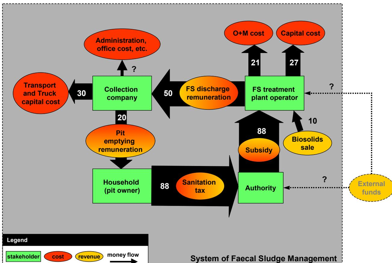
**Figure 6:** Emptying company and pit holders are remunerated for FS delivery. Remuneration and FS treatment are subsidised by the authority via a sanitation or similar tax.
