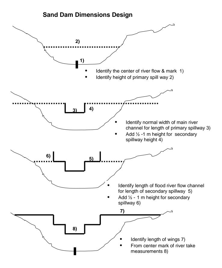
Figure 2. Summary of steps taken to determine sand dam dimensions.
