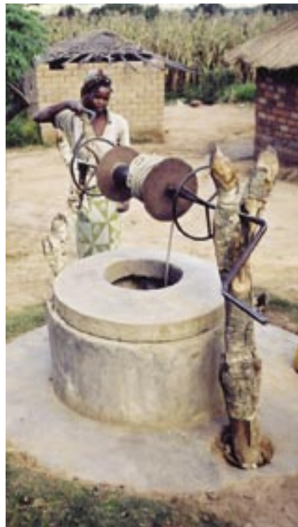
Before and after: Low-cost lifting devices such as windlasses have improved water supply.
