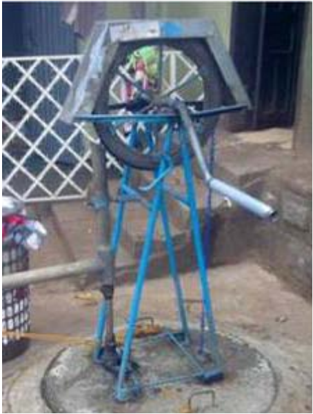
Figure 0-4 Rope pump in family yard in Chencha, used for all domestic purposes
