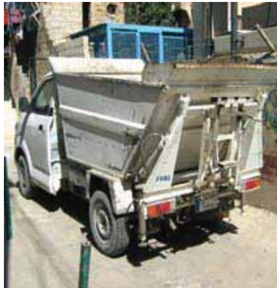
UNRWA dumper collecting solid waste in Mieħ Mieħ AA
