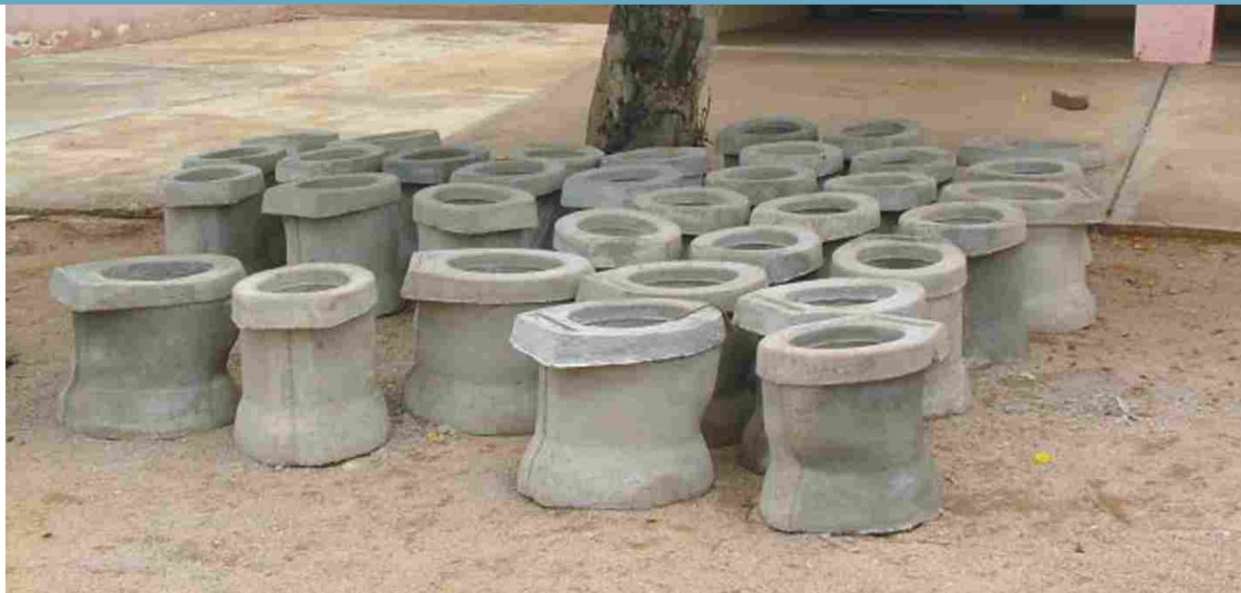
VIP Pedestals built by the local builders
