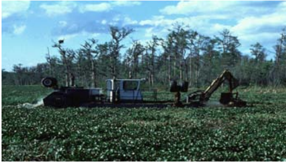
Plate 1.1: Mechanical Cutter for Water Hyacinth
