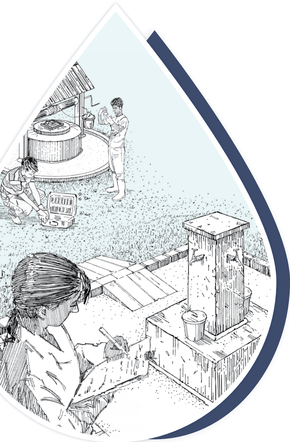
Sanitary inspection and water quality testing being carried out at a public tapstand and dug well. See Fig. A4.2 for additional small water supplies covered by sanitary inspection tools.
