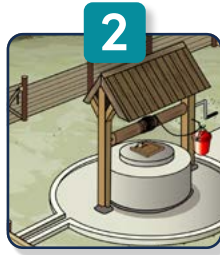
2 Dug well with a windlass
