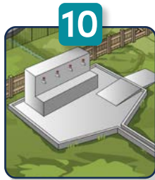
10 Piped distribution: tapstand
