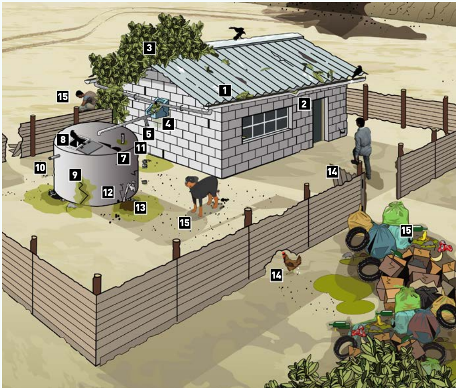
Fig. 4.2 • Excerpt from the SI form risk factor illustration for rainwater collection and storage
