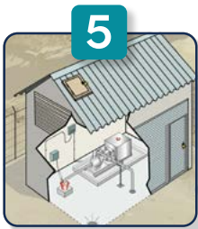
5 Borehole with a motorized pump
