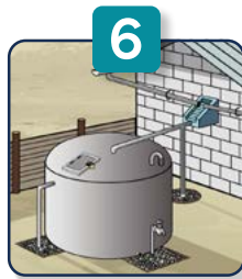
6 Rainwater collection and storage
