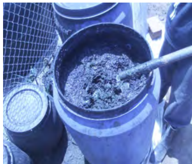
Faecal sludge mixed with non biodegradable waste.
